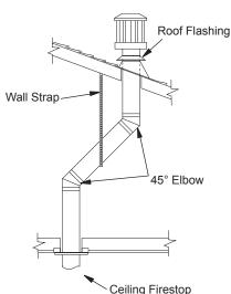
Figure 16 - Offset with Wall Strap and 45° Elbows
